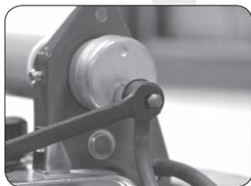
5.3.1 Disassemble the one-way valve.
