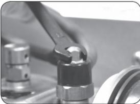
5.7.4 When install back the one-way valve, please do not install it too tightly, otherwise if the air pressure could not get through will have problem.
