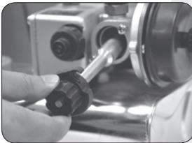
3.2.7 Install back swirl pole in appropriately, when fastening screws make sure use strength in balance.
