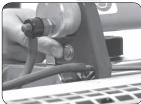
5.1.1 Take down high voltage cap put down on carburetor as photos showed, then press down ignition button
