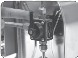
After machine start up for 20 seconds until machine work stably, turn chemicals valve to "ON" position, start spraying fog.
