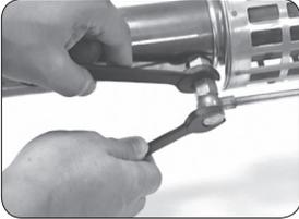
3.4.1 Disassemble the nozzle, do not lose copper gasket.
