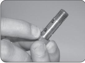
5.8.2 Check whether the screw hole is blocked, clean it.
