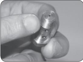
5.8.3 Check whether the screw hole is blocked, use thin wire get through it.
