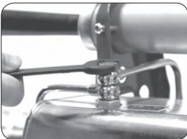
5.8.5 Install back appropriately, if too tightly will broken the screw.
