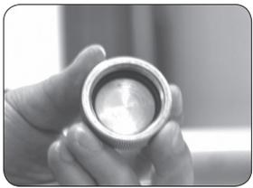
1.4 Use white funnel fill chemicals solution into chemicals tank, only fill 4/5 full chemicals tank capacity will be ok, check whether the O-Ring of fuel tank lid is in good condition? Then, tighten chemicals tank lid appropriately.
