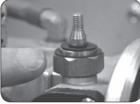
5.7.2 Check whether the gasket is broken or deformed, if has, change, the photo showed is ok.
