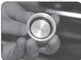
5.4.2 Check O-Ring, if it is broken or deformed, please change it, when install back fuel tank lid to fuel tank, please do not install it too tightly.
