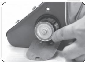
5.2.1 Open battery tube cover, check battery.
