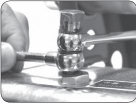
5.8.4 After clean, install back in appropriately, do not lose the 3 pcs red gasket.
