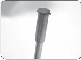
3.2.4 Make sure the two needles is in symmetrical at the two sides of the swirl pole.
