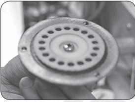
3.1.9 Watch whether the diaphragm could move freely inside the groove of the diaphragm fixed plate, do not install it too tightly.
