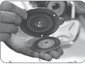
3.1.7 As photo showed, make the valve plate point to the groove of the diaphragm fixed plate, put onto it, makes sure the diaphragm could move freely inside the groove.
