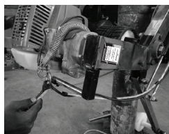
ATTACHING CABLE AND ROPE TO BRAKE LEVER
