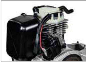
Engine with 4-stroke technology and overhead valves (OHV).
