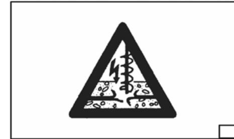
**WARNING – Striking a hard object in the earth with the turning auger and the resulting slowing or stopping of the auger creates reactive forces. The transfer of rotational (reactive) forces can cause the auger power head and handles to rotate suddenly in a counterclockwise direction and can result in loss of control or cause the handle frame to hit the operator or throw him to the ground, resulting in serious injury**
